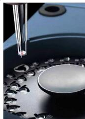
**Figure 1.** Pictures of (a) Auto Q2000 DSC (left) and (b) DSC auto-sampler in RPI Polymer Center.
