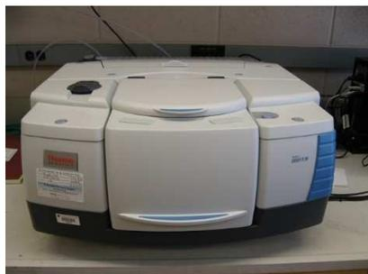
Students will use Thermo-Scientific iS50 FTIR spectrometer in RPI Polymer Center to analyze their polymer samples typically in a form of films. FTIR spectrum will be taken in the wave number range from 4000 to 700 cm<sup>-1</sup>.
