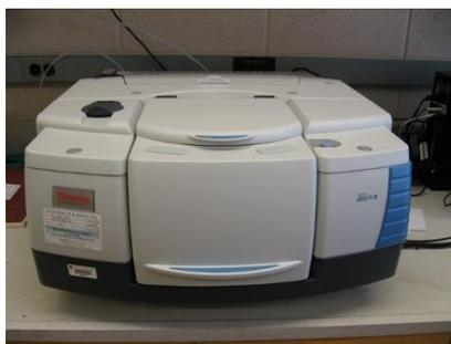
Students will use Thermo-Scientific iS50 FTIR spectrometer in RPI Polymer Center to analyze their polymer samples typically in a form of films. FTIR spectrum will be taken in the wave number range from 4000 to 700  $\text{cm}^{-1}$ .
