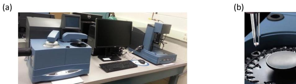
**Figure 2.** Pictures of (a) Auto Q2000 DSC (left) and (b) DSC auto-sampler in RPI Polymer Center.
